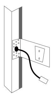
\*\* To switch between mounting to the LEFT or RIGHT of a window frame. Remove the VESA mount, then remove the 2 x M6 nuts and flip adaptor plate to suit.
